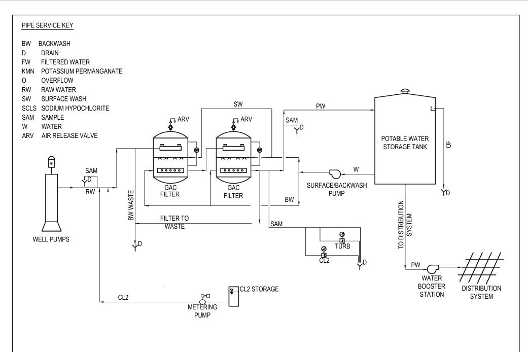
Figure 4-2 Acorn Environmental Scotts Valley Rancheria Water and Wastewater Feasibility Study Preliminary Process Flow Diagram
