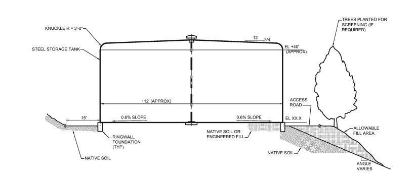
Figure 4-3 Acorn Environmental Scotts Valley Rancheria Water and Wastewater Feasibility Study Typical Water Storage Tank
